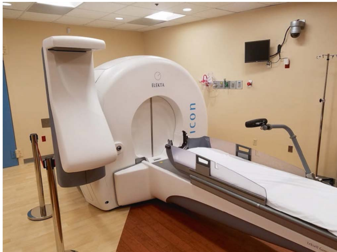
Fig. 2.1 Elekta GammaKnife® Icon unit, which collimates 192 Cobalt-60 sources to deliver multiple beams simultaneously
